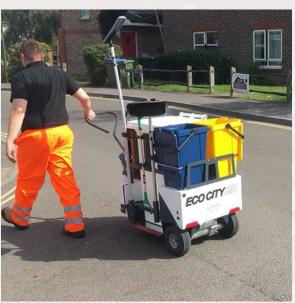
Careful attention has be paid to the type of environment the Eco City Bin will be used in and as such the unit comes as standard with an operating LED light, horn for attracting attention, permanent flashing LED's and reverse beeper.
