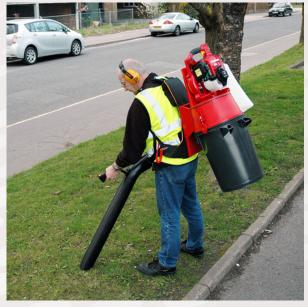
This machine can hold up to 35 litres of rubbish which is collected through either a 5" or 4" vacuum hose (3" vac hose is used for collecting dog faeces). This now allows the operator to go literally anywhere and collect rubbish.
