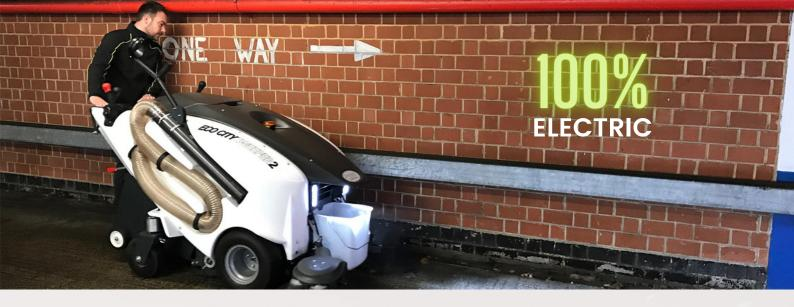
The Eco City Sweeper 2 is also incredibly versatile because it can be used both as a walk behind machine, and a ride-on machine with the addition of a chariot, this offers the possibility to drive for long distances. It is also equipped with a wander suction hose for vacuuming bulky waste reaching narrow spaces such as flower beds, side benches, etc.
