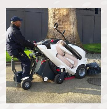
The Eco City Sweeper 2 is powered by a 24v 320 amp hour battery pack providing a 10 hour run time with an overnight charge.
